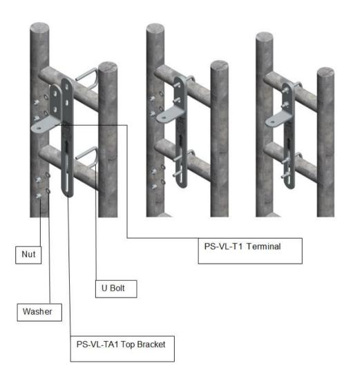
PS-VL-ETA1 Ladder Extension installation is done with U bolt, braket, washer and nut. The installation is completed with Ø19 mm wrench.
