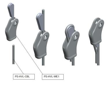
PS-HVL-WE1 Wire Ending installation is done with bolt washer and nut. The installation is completed with Ø19 mm wrench.
